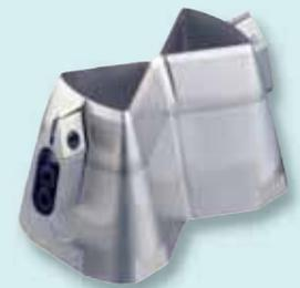
The cutting die for our label example is manufactured with a 7 mm long middle bridge positioned between the prints. The two ready cut label rows run separated onto the delivery tray. This method offers simplified handling, double throughput of the machine and saving on guillotining cost.
