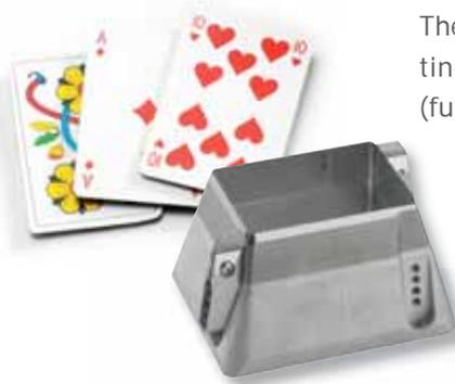
The example illustrates a die for cutting the complete outer contour (full-cut) of playing cards. The waste slitters are screwed on to the die.
