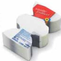
This example shows a die for the full-cut of a plastic foil in-mould label. The cut is made using counter-pressure. The counter-pressure matrix – shown in the middle – exactly matches the die form. The movable matrix inside the die uses compressed air to supply the counter-pressure during the cutting process.
