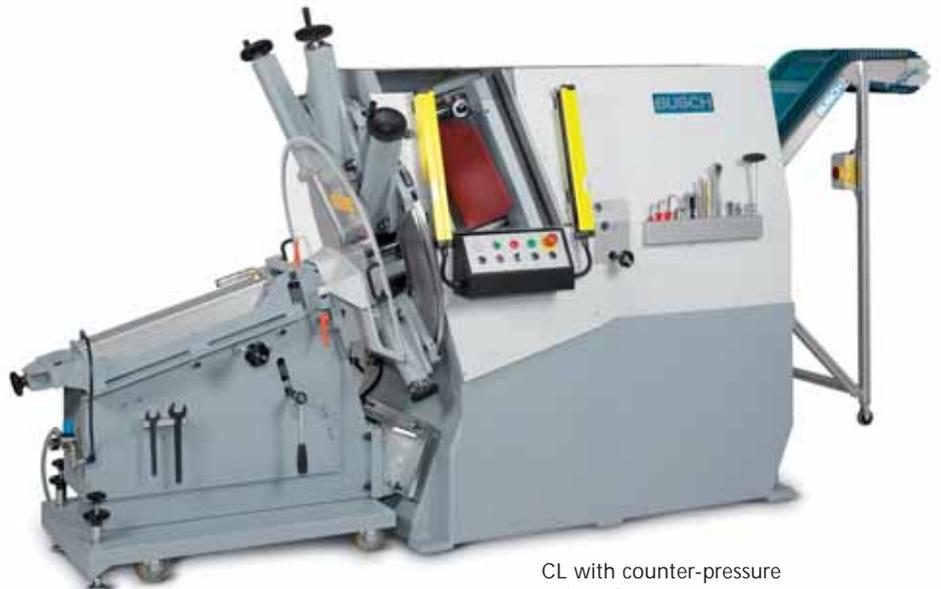
CL with counter-pressure unit and waste conveyor
