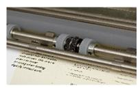
Built in perforating wheel which is easily engaged for in-line perfing.
