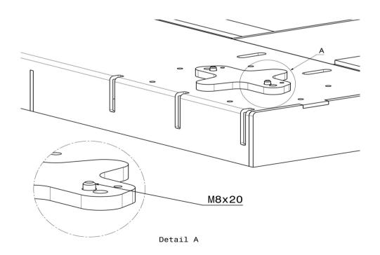
• Place the quick-change-system base on the frame of the heat press - all black hand screws are pointing forwards and the hooks for taking up the exchangeable base plates are pointing upwards.
