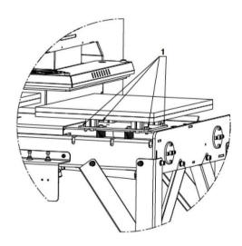
• Remove the base plate of the TPD7 PREMIUM and loosen the pre-mounted adapter plate.
