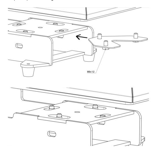
Place the quick-change-system base on the frame of the heat press - all black hand screws are pointing forwards and the hooks for taking up the exchangeable base plates are pointing upwards.
