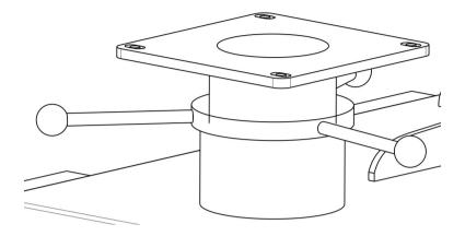
• Loosen the threaded bolts at the adjustment ring below the base plate.
