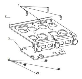
• The quick-change-system has to be mounted onto the socket of the TPD7 PREMIUM and tighten all screws.
