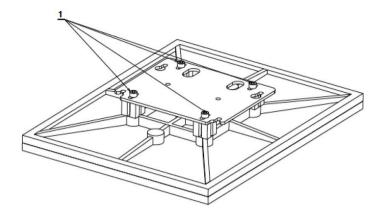
Mount on the Beam-Adapter below the base part of the quick-change-system by using included screws
