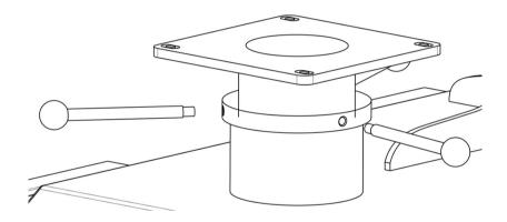
• Place the quick-change-system base at the corresponding position and stick the appropriate screws from upwards through the holes. Tighten the screws and washers.
