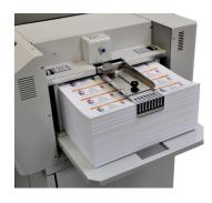
The new Zip-21A cutter/slitter is the deep pile, Air fed version of the original Zip21C designed to cut business cards & other multiple-up products produced from a range of different printing methods. The Zip21A is faster than the Zip21C, producing 18,500 cards per hour and comes mounted on a stand which houses the extra large waste container required for such quick operating speeds.
