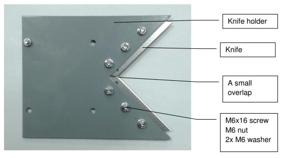
Adjust the cutting plate as it is described in the previous section. Do not forget to mount back the transparent plastic safety guard.
