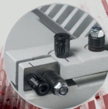
92 advance , scaled swinging / tilting adjustment for massive back gauge
